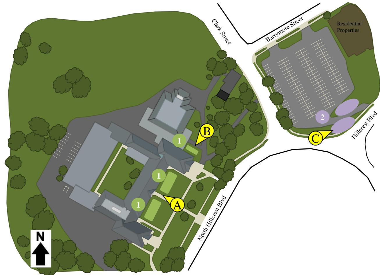
**1 BIORETENTION SYSTEMS:** Bioretention systems could be installed in the turfgrass areas where downspouts can be disconnected on either side of the entrance as well as on the side of the school. A bioretention system will reduce runoff and allow stormwater infiltration, decreasing the amount of contaminants that reaches catch basins.
