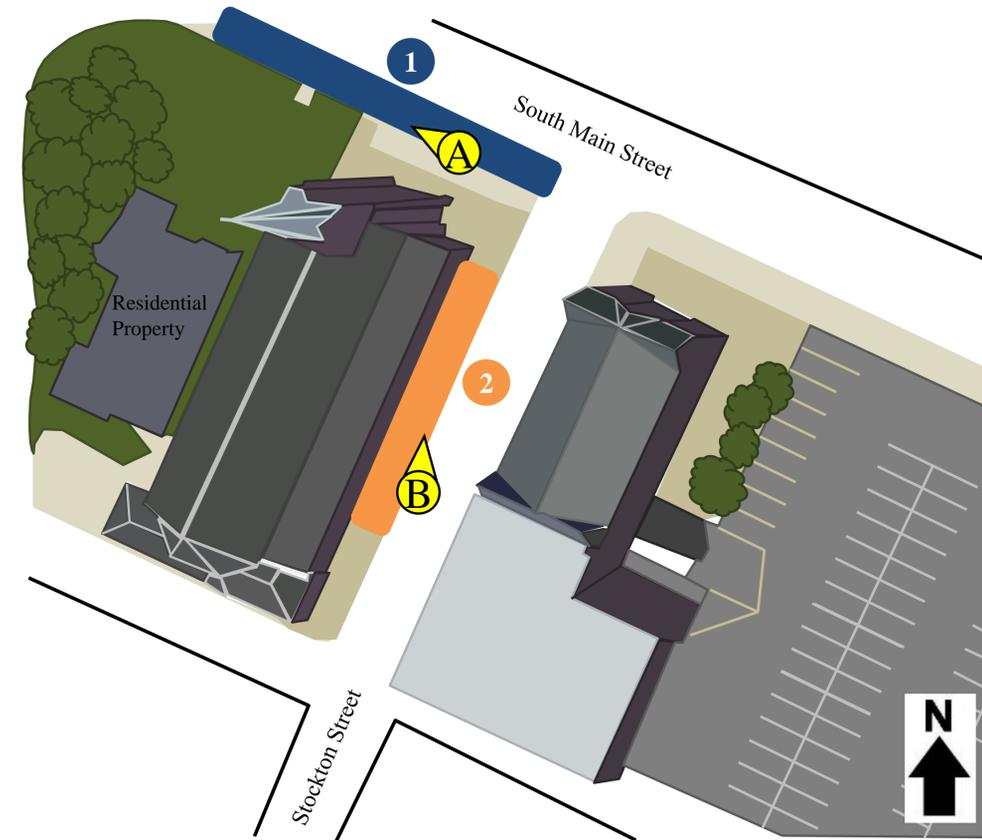
**1 TREE FILTER BOX:** A tree filter box could be installed along the sidewalk in the front of the church to catch and treat the first flush of stormwater prior to discharge into the stormwater system.
